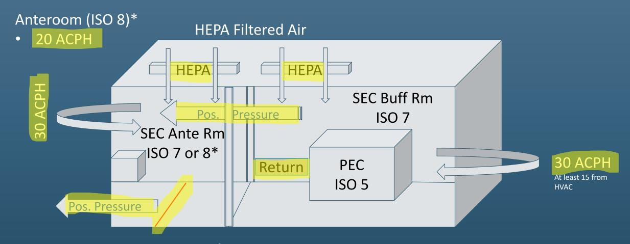
\*Note: Anteroom must be ISO 7 w/ 30 ACPH if connected to negative pressure HD ISO 7 Buffer Room
